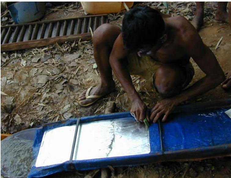
Figure 5. Scraping Mercury off Metal Flume
