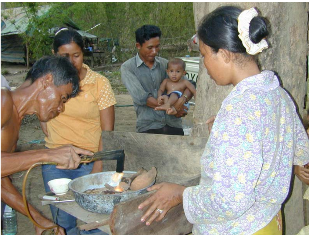
Figure 6. Heating Amalgam to Volatilize Mercury and Recover Gold
