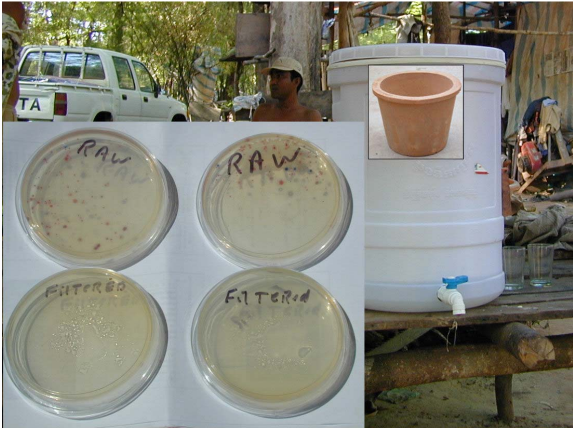
Figure 15. Ceramic Water Filter Removed Bacteria from Well Water
