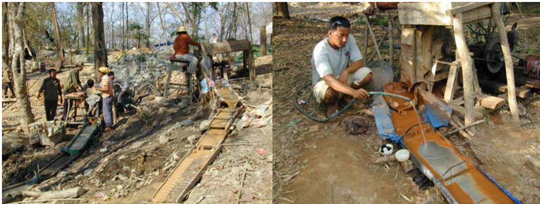
Figure 3. Flumes for Gold Recovery (hose at right was used to reveal mercury)
