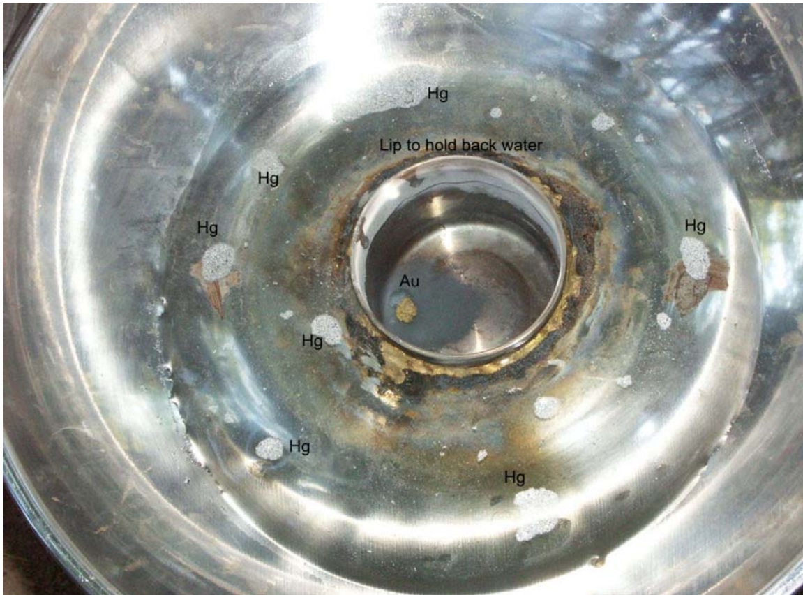
Figure 12. Retort After Separation of Mercury and Gold
