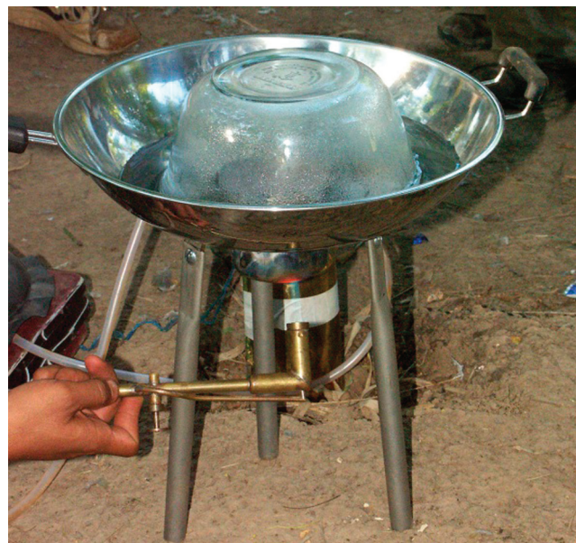
Figure 3. Frying Pan Retort (photo T. Murphy). The retort enables separation and recovery of mercury from gold amalgams without exposing the miner to mercury fumes.
