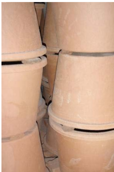
Figure 4.9 Filter elements stacked in kiln
