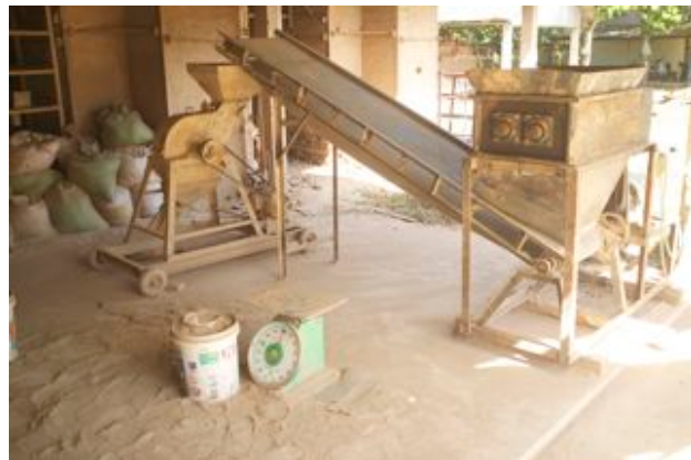
Figure 4.3 Brick crusher machine (new method)
