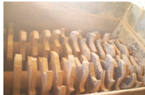
Figure 4.4 Counter-rotating teeth of machine capture bricks for crushing
