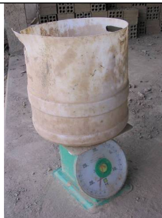
Figure 4.7 Scales for weighing out clay powder from the hammer mill.
