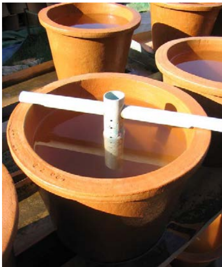
Figure 4.18 T-piece measuring flow rate
