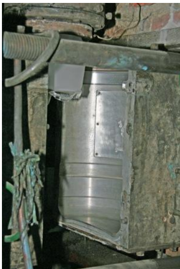
Figure 3.2 Blow mould for RDIC plastic receptacle
