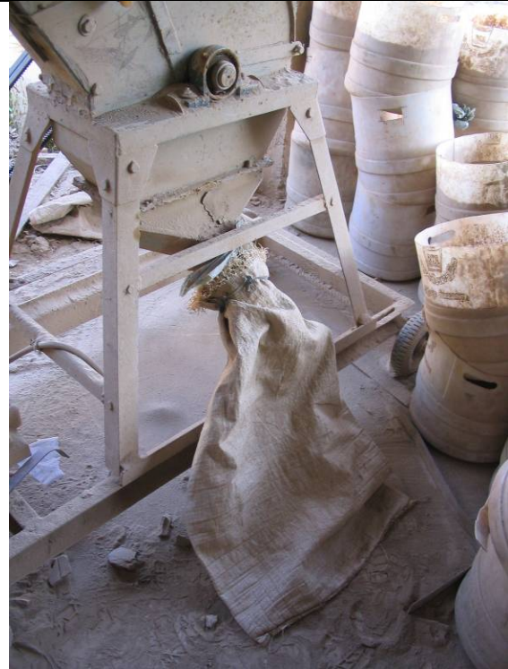
Figure 4.6 Hammer mill discharge with rice sack attached
