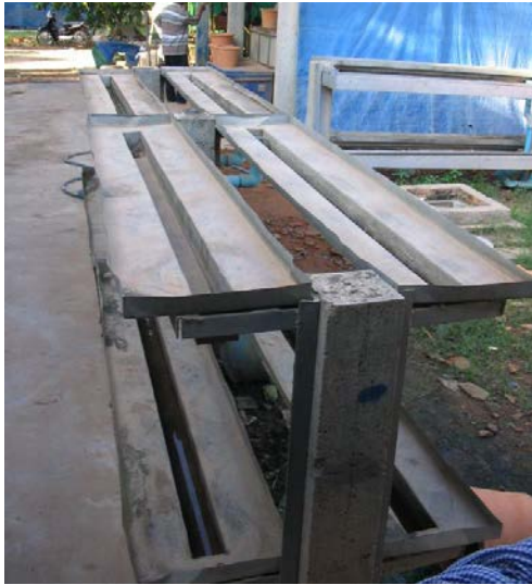
Figure 4.16 Filter rack for flow rate test
