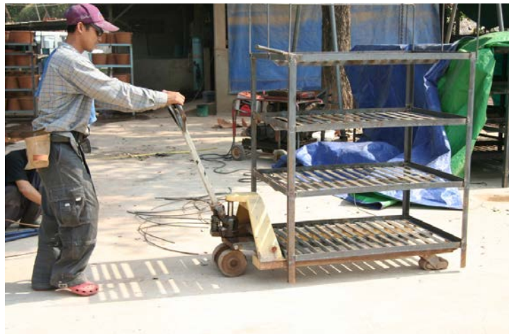
Figure 4.4 Manual pallet trolley used to shift drying racks
