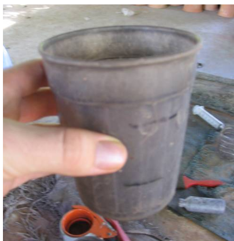
Figure 4.20 Cup for measuring silver nitrate solution (note 2 levels marked)
