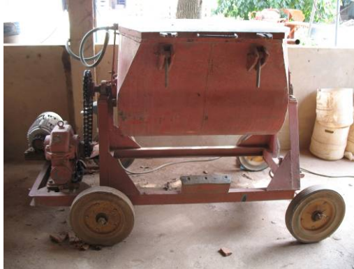
Figure 4.10 Clay Mixer - during operation
