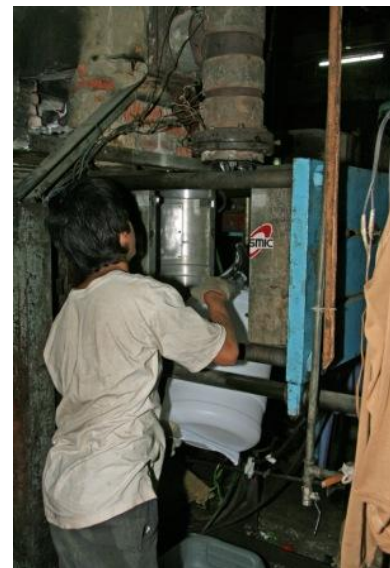
Figure 3.4 Removing moulded receptacle from mould
