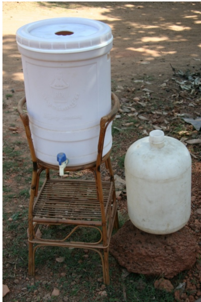
Figure 4.31 Ceramic Water Filter System with modifications to allow 20L container to be inverted to provide additional storage for pre-filtered water.
