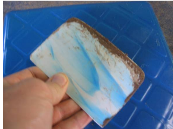
Figure 4.20 Plastic scraper for smoothing filter elements
