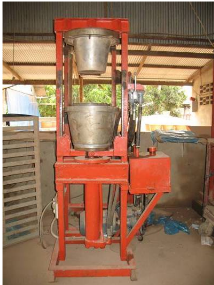
Figure 4.14 RDIC's hydraulic press
