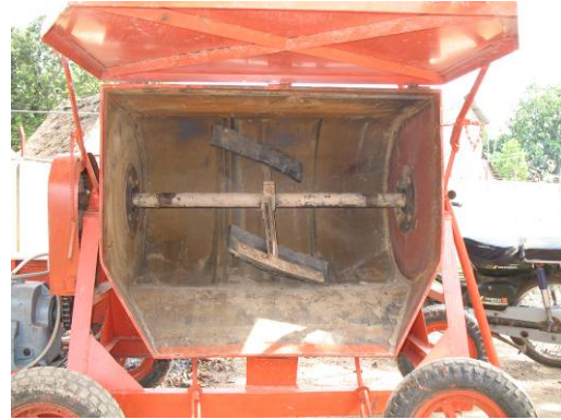
Figure 4.11 Clay Mixer - open for emptying
