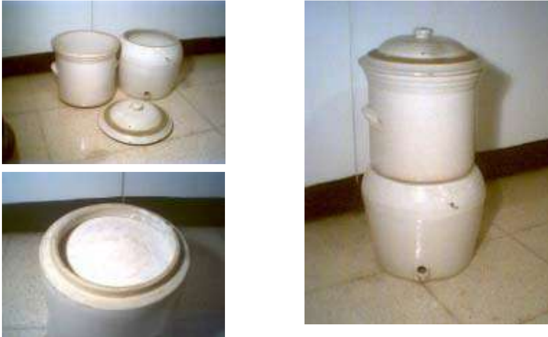
Figure 3-2. 100-year-old Spanish ceramic disk filter
