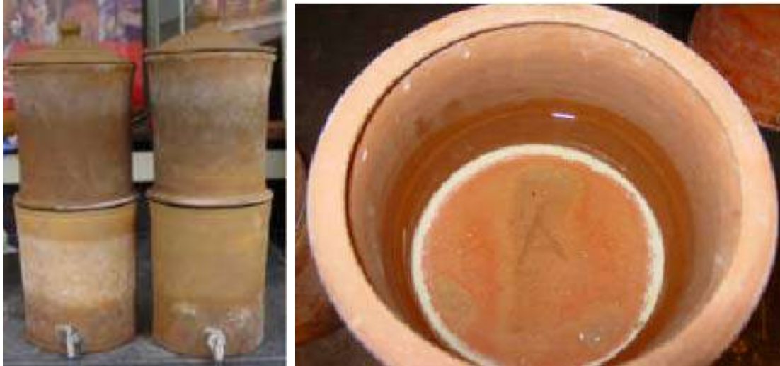
Figure 3-4. Terracotta Ceramic Disk Filters
