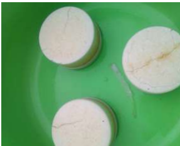
Figure 3-39. Ceramic candles with cracks on the surface
